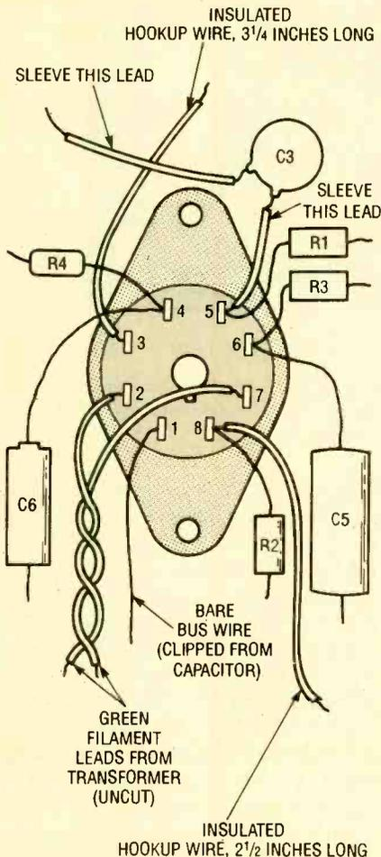
Fig. 5. Before mounting the tube socket on the board, wire C3, C5, C6, R1-R4, and the three connecting wires to the socket.
