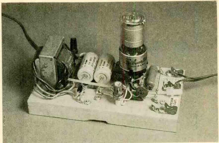
The Radio Transmitter, with its baseboard-mounted components, which is representative of the construction technique used during the 1920's, is patterned closely after the phono transmitters of yesteryear.
